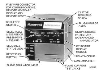
Fig. 1. Keyboard Display Module and sequence status LEDs.
