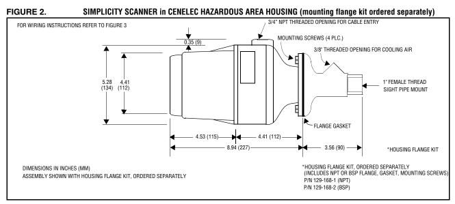
**NOTE:** All models of the Simplicity 65UV5-1004 CEX flame scanners are housed within an ATEX approved housing for application in Exd IIC T6 hazardous rated environment. In addition the ATEX housing is designed to meet the requirements of IP66 (NEMA 4X).
