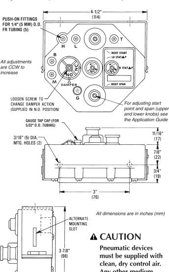
Any other medium (e.g., oil or moisture contamination) will cause the device to fail. \*(These instructions do **not** apply to the CSC-3014 or the CSC-3501/3505; see their separate Installation Guides.)
