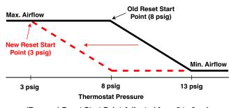
(Reverse) Reset Start Point Adjusted from 8 to 3 psi
