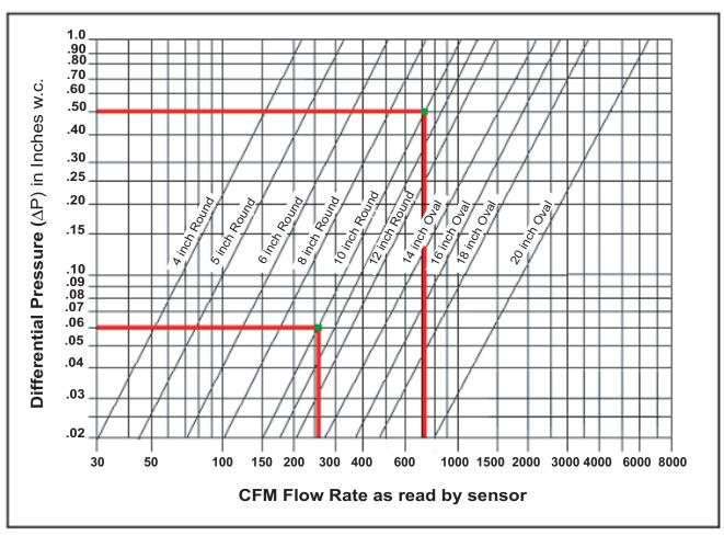
VAV Airflow Rate by Duct Size
