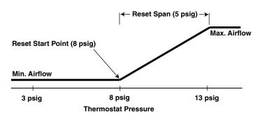
NOTE: Reset span is the pressure change at "T" above the reset start point that causes the flow setpoint to move from one extreme to the other. In a direct reset application, the flow setpoint will change from minimum to maximum flow above the start point. In a reverse reset application, the reset will change from maximum to minimum flow above the start point.
