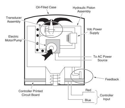
Figure-17 MP-5400 Series Actuators.
