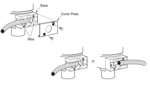
Figure-7 Flexible Conduit Installation to Either Side of Actuator.
