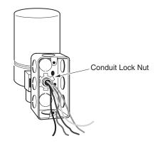
Figure-12 Attachment of Conduit Box to Threaded Adaptor.
