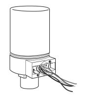
Figure-5 Wire Leads Connection (No Conduit).
