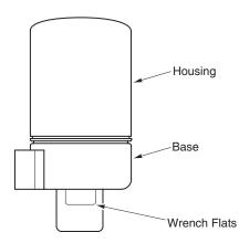
Figure-3 Housing and Base Location.
