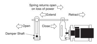
Figure-14 Dampers Open When Actuator Extends (Spring-Returns Closed on Power Loss).
