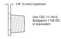
Figure-10 1/2" Conduit Bushing.
