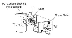
Figure-11 Conduit Bushing and Cover Plate Installation.
