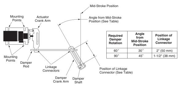
Figure-15 Actuator/Damper Mounting.
