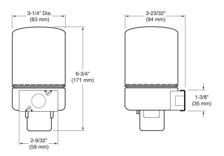
Figure-19 Actuator Dimensions.
