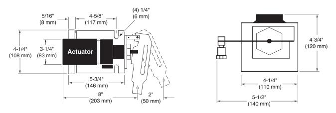
Figure-18 Damper Linkage Assembly Dimensions.
