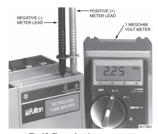
Fig. 10. Flame signal measurement.
