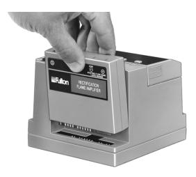
Fig. 5. Installing Plug-In Flame Signal Amplifier.
