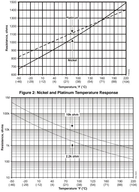
**Figure 3: Thermistor Sensor Response**
