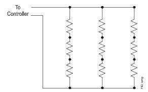
Figure 4: Nine-Sensor Series-Parallel Wiring
