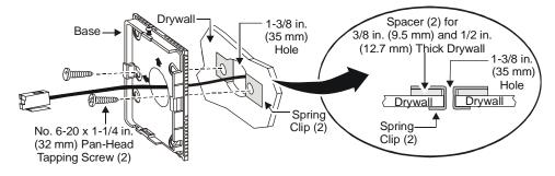
Figure 5: Surface Mounting to Drywall
