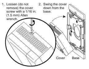
Figure 1: Removing the Cover from the Base
