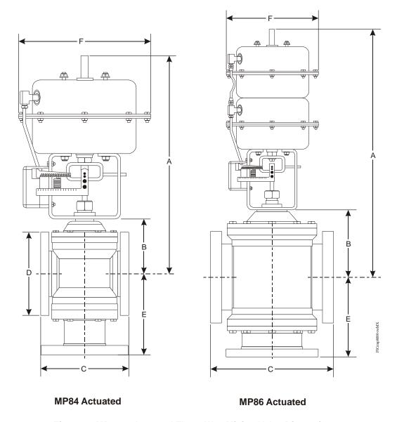
Figure 3: MP8000 Actuated Three-Way Mixing Valve Dimensions (See Table 3.)
