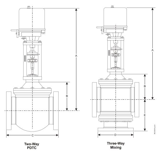
Figure 6: VA-610x Actuated Valve Dimensions (See Table 6.)
