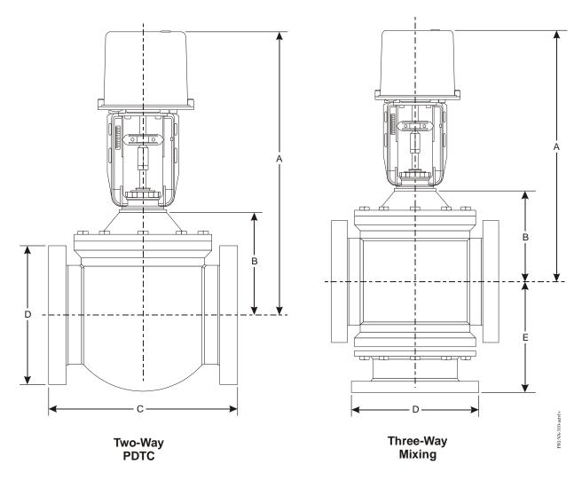
Figure 5: VA-310x Actuated Valve Dimensions (See Table 5.)
