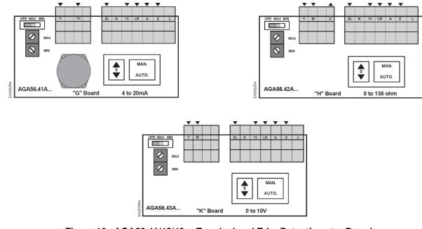
Figure 10. AGA56.41/42/43... Terminal and Trim Potentiometer Boards.
