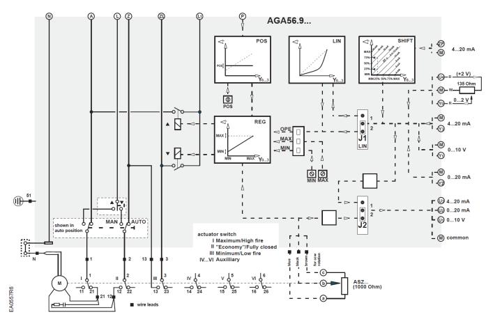
Figure 11. Basic Functional Diagram of AGA56.9...
