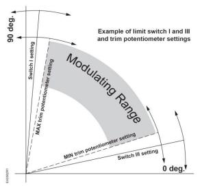
Figure 13. Switch Cam and Trim Potentiometer Setting.
