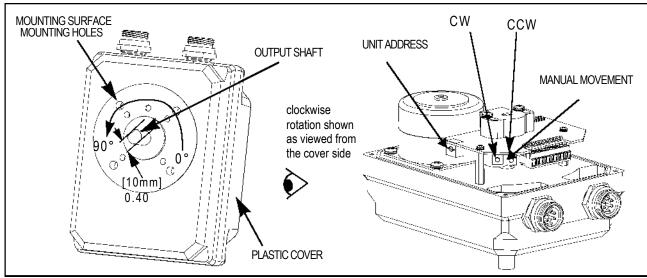
WARNING - DO NOT USE THE MANUAL MOVEMENT SWITCHES ON THE SERVO MOTORS DURING AUTOMATIC OPERATION OR THE FIRING CYCLE OF THE BURNER. USE OF THE MANUAL MOVEMENT SWITCHES OPERATES THE SERVOMOTORS INDEPENDENT OF THE PPC4000 CONTROL AND COULD RESULT IN AN OFF-RATIO CONDITION IF OPERATED DURING AUTOMATIC OPERATION OR THE FIRING CYCLE
