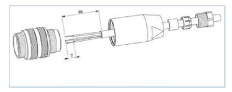
As shown above the cable strip length is specified at 30 mm (1.2 in) and each wire strip length is 7 mm (0.275 in).
