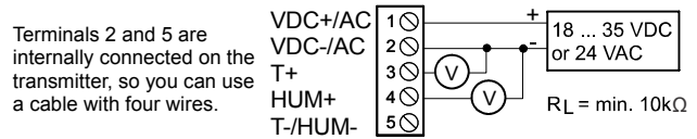
Figure 11: HE-68P3-0N000 Wiring
